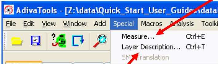
Measure provides a tool allowing the user to drag a line anywhere on the screen and a total distance from start to end is displayed in the status bar at the bottom of the Adiva Graphical Interface.
